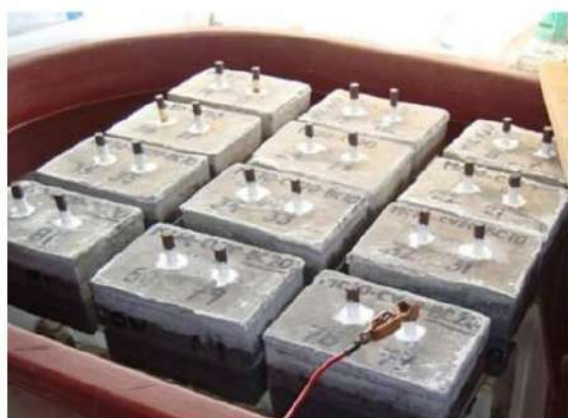
Fig. 1. The exposure conditions of the reinforced prismatic specimens.
