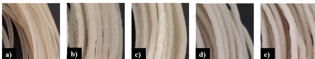
Figure 1. Filaments of different formulations: a) TPS; b) TPS/Fiber; c) Hybrid with 3% of calcium carbonate; d) Hybrid with 5% of calcium carbonate; e) Hybrid with 7% of calcium carbonate.
